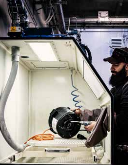
Compressed air connection and blow gun nozzle. Suction hose for easy cleaning inside the cabinet.
