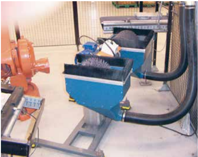
Robot deburring for telecom parts
