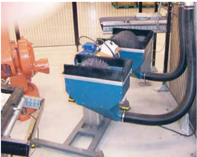
Robot deburring for telecom parts
