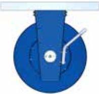
Hose guide installed upwards.
