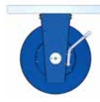
Hose guide installed upwards.
