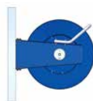
Hose guide installed outwards.
