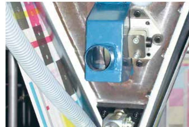
Suction casing mounted on slit knife in printing press
