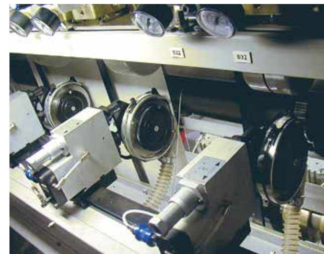
Suction casing mounted on slit knife in printing press
